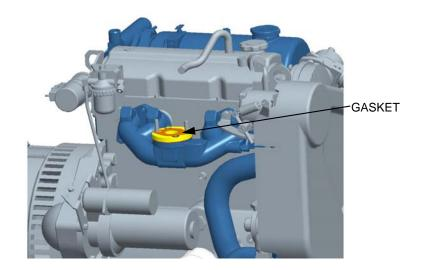
10. Place new carburetor (P/N 52563) on top of gasket.
